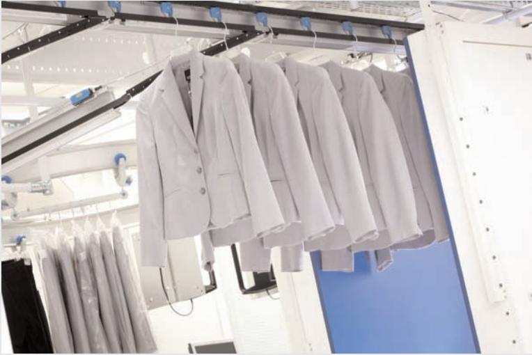
Figure 3: Hanging sorter with tagged articles of clothing Source: Metro AG
